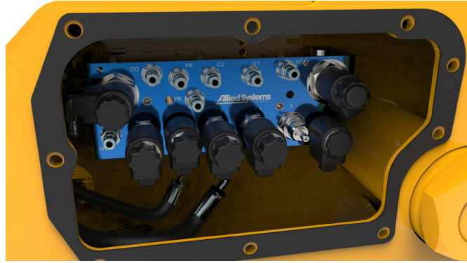
Figure 2-18 Remove Control Valve Cover Plate
